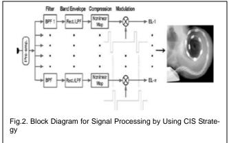
In the figure 2, the speech and other sounds are represented in a simpler manner. In order to represent the fundamental frequencies of speech sounds the cut-off frequency of the LPF is set at greater than or equal to 200 Hz in each envelop detector. As of now, 4 to 24 channels are used in CIS strategy to process speech and other sound signals [5] [6].
